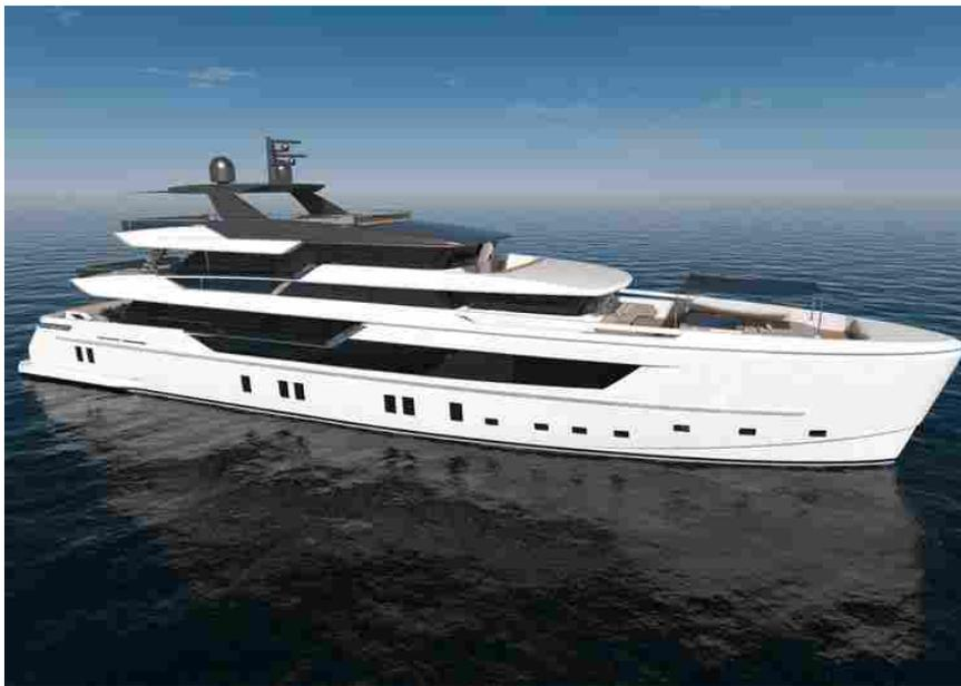
Power to the vessel is provided by twin MTU 12V 2000 M96L 2636 hp diesel engines, enabling her to reach a top speed of 21 knots and cruise comfortably at 18 knots.
